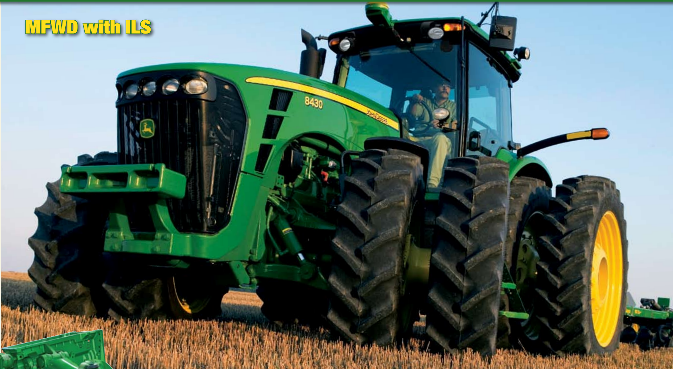
The 1500 Series MFWD lets you add duals to your front axle for added load-carrying capacity, traction, and flotation.
