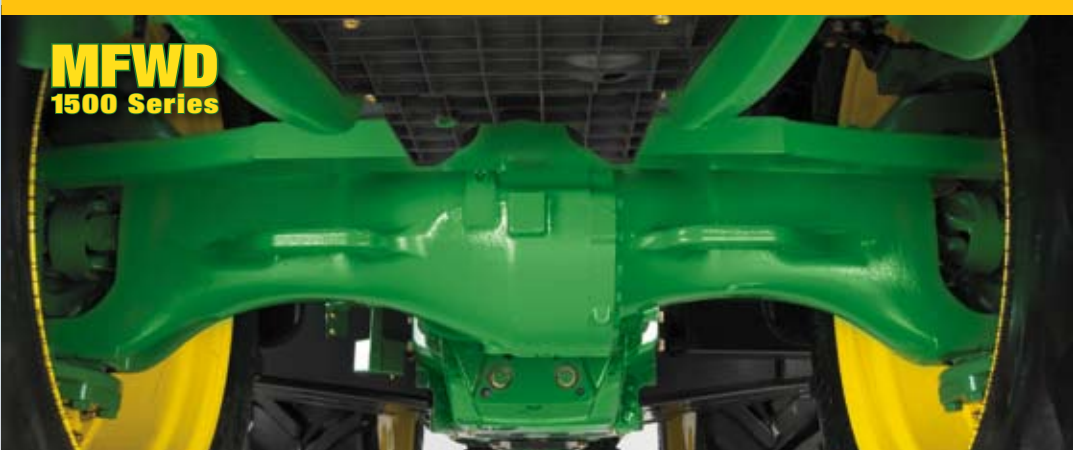
The 1500 Series MFWD lets you add duals to your front axle for added load-carrying capacity, traction, and flotation.
